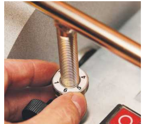
▲ The tool post has the standard Tormek fine-height adjustment for tweaking the angle
